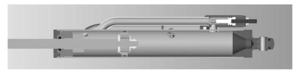
The illustration above show piston is inside the bypass circuit. This is evident because the tube starts where the bend is welded to the body, and ends where the bypass unit is welded to the body.
